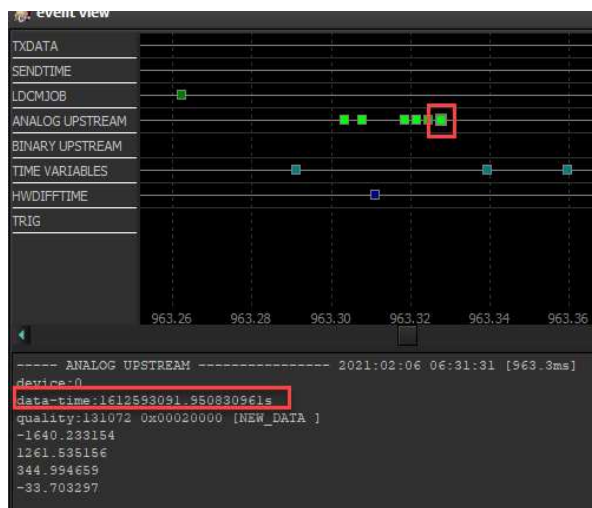
Figure 8. Details of relay-to-relay communication message received at Malin, 950.83ms
