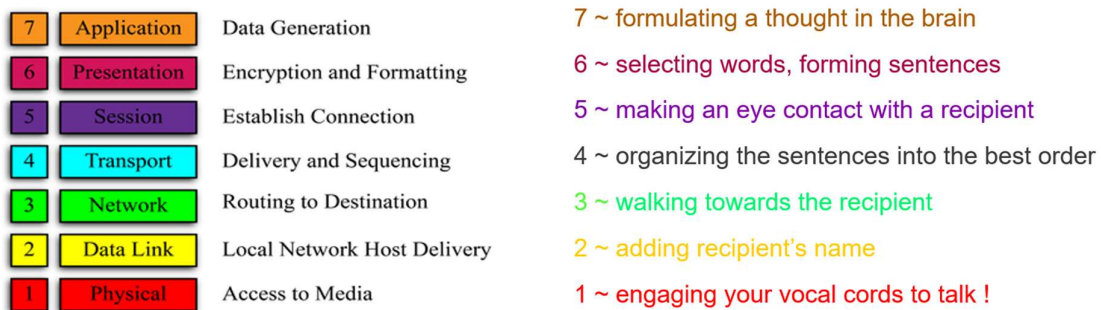
Figure 2 Explaining 7-Layer OSI model using human communication analogy
