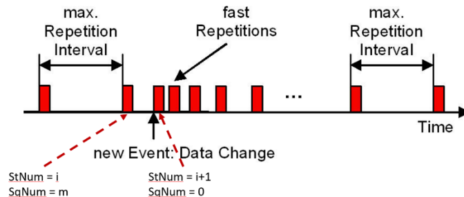
Fig. 2 GOOSE repetition mechanism
