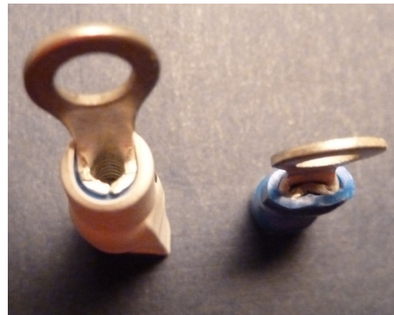
Fig. 19. Photograph of the Actual Ring Lug (Left) and Example Crimped Lug (Right)
