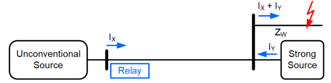
Fig. 2. External fault behind the remote terminal.
