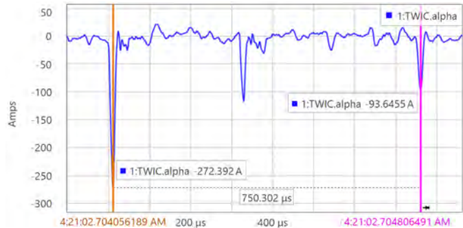
Fig. 30. West Shackelford C-phase alpha-mode current TW arrival times: t_1 = 2.704056189 s and t_4 = 2.704806491 s.
