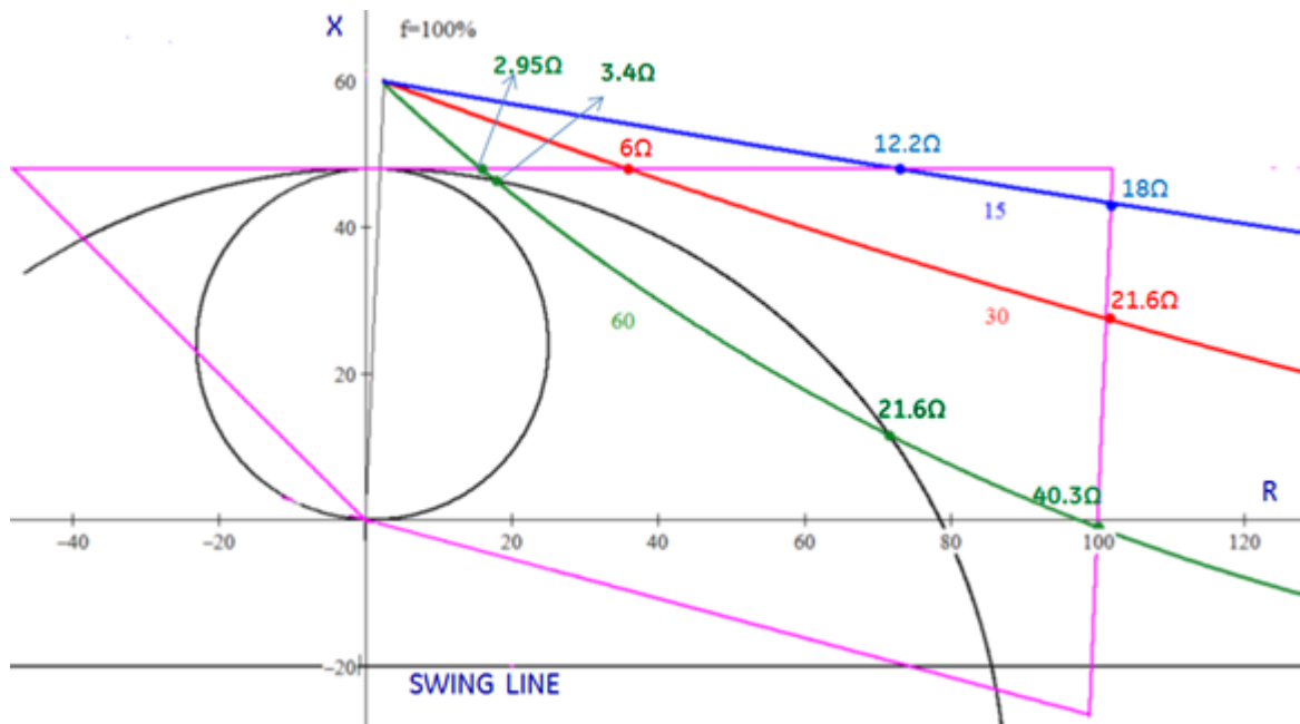
Figure 26: Calculated Relay Reaches, Weak Source, Swing Angles of 15^\circ , 30^\circ and 60^\circ , Remote Terminal Fault.
