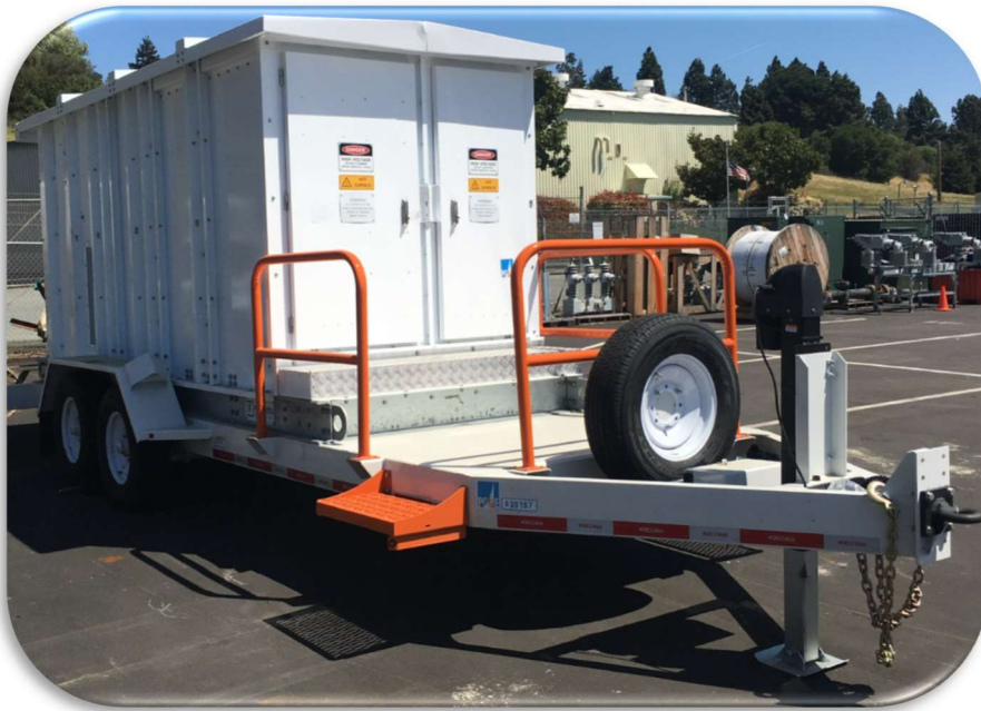
Figure 6 Test trailer with high voltage resistor bank up to 25,400 ohms
