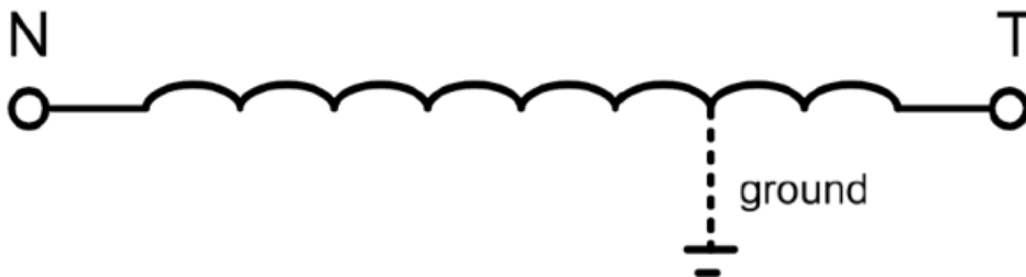
FIGURE 8. Fault Location with Respect to Generator Neutral
