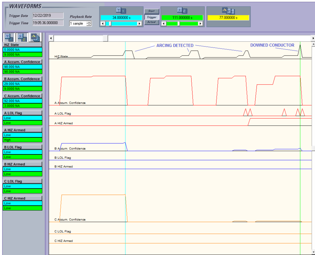
Figure 2. Hi-Z oscillography for a True Downed Conductor Operation of F60 Hi-Z element.
