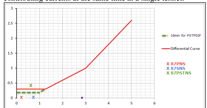
Fig 8: 1p.u Negative Sequence Internal Fault
