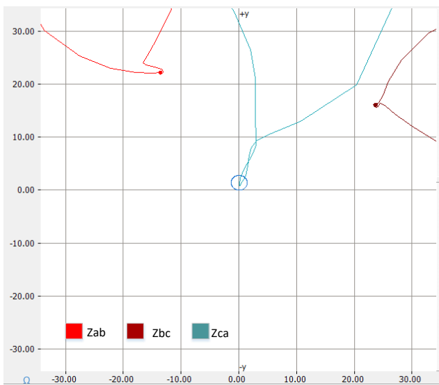
Fig. 9. Impedance diagram for a SLG fault at 0% of the interconnection line (residual voltage compensated)
