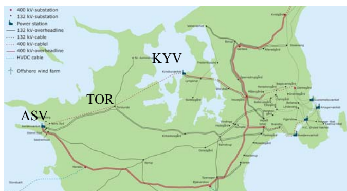
Fig. 7. The planned 400 kV ASV – TOR – KYV cable line in the Eastern Danish grid (courtesy of Energinet.dk).
