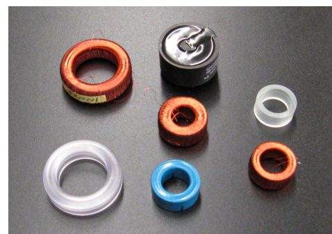
Fig. 2. Conventional CT and the Rogowski coils with conventional CT components in the middle (core, core with secondary, and completed CT assembly).
