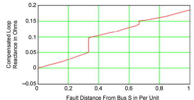
Fig. 11. Compensated loop reactance ( k_0 = 0.66/\Omega^0 ) in ohms for cross-bonded cable
