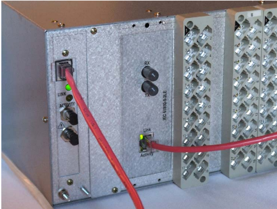
Fig. 8 IED Station and Process Bus interfaces
