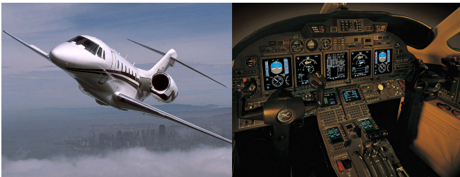
Fig. 2. Aircraft dual primary systems of one manufacturer: same engines, same radios, same air-data computers, and same flight management systems. Photos courtesy of Cessna Aircraft Company.
