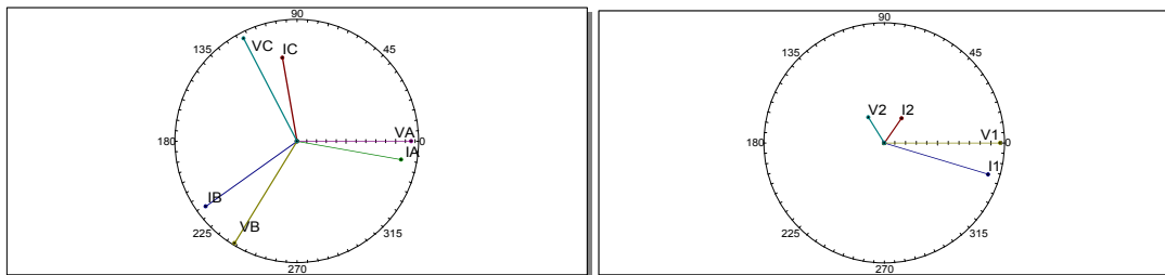
Figure 6 Fault (Cycle 10) Phase Voltages and Currents (left), Symmetrical-Components (right); Referenced to V1 at Zero Degrees
