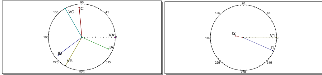
Figure 4 Prefault (Cycle 5) Phase Voltages and Currents (left), Symmetrical-Components (right); V1 Referenced to Zero Degrees
