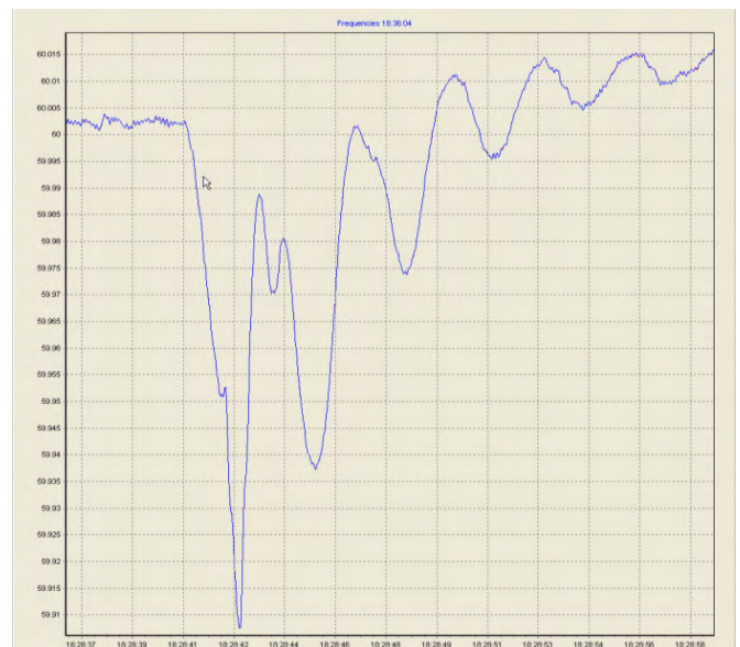
Fig. 14. Synchrophasor Data Plot Showing Frequency Excursion at Distribution Voltages
