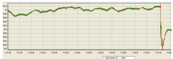
Fig. 15. BPA Synchrophasor Data Plot Frequency Excursion at Transmission Voltages
