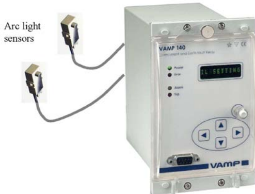
Figure 6. An overcurrent relay with intergrated arc protection.
