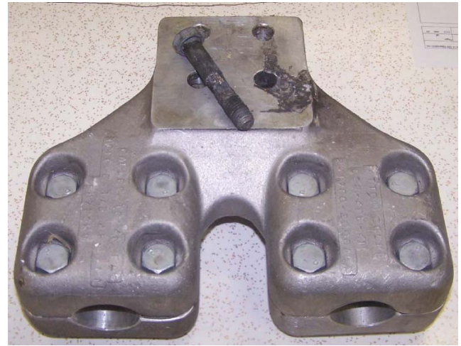
Figure 10 Damage to the Connector Due to Loose Connection
