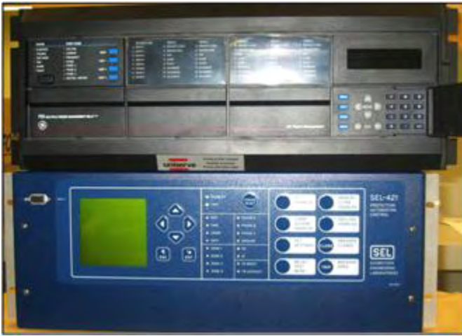
Fig. 32. Third generation (numerical) protection relay.
