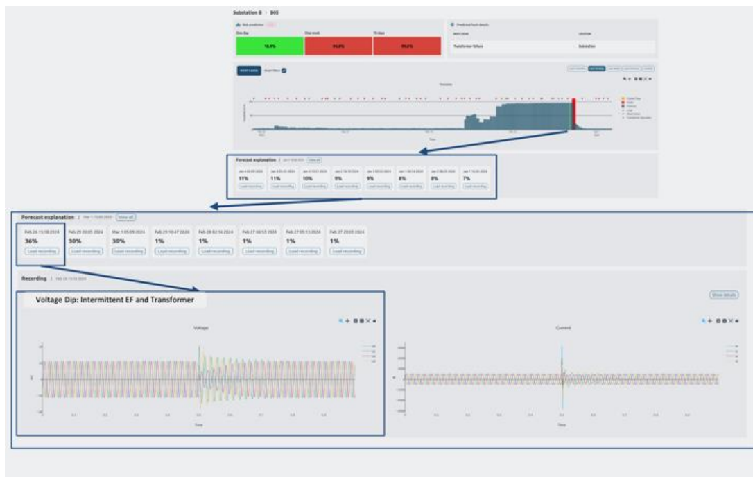
Figure 11. Example of the XAI module providing the reason for a high fault risk estimation based on 10 anomalies that are pre-indicators of evolving faults.
