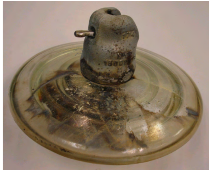
Fig. 1. A flashed insulator bell identified by a patrol crew: UB of Bonneville Power Administration [3].
