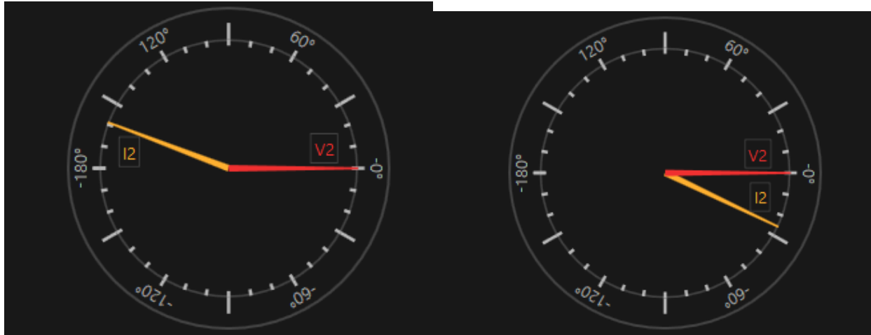
Figure 6. Phasor diagrams (V2 and I2) plotted from the oscillography of event recording relay
